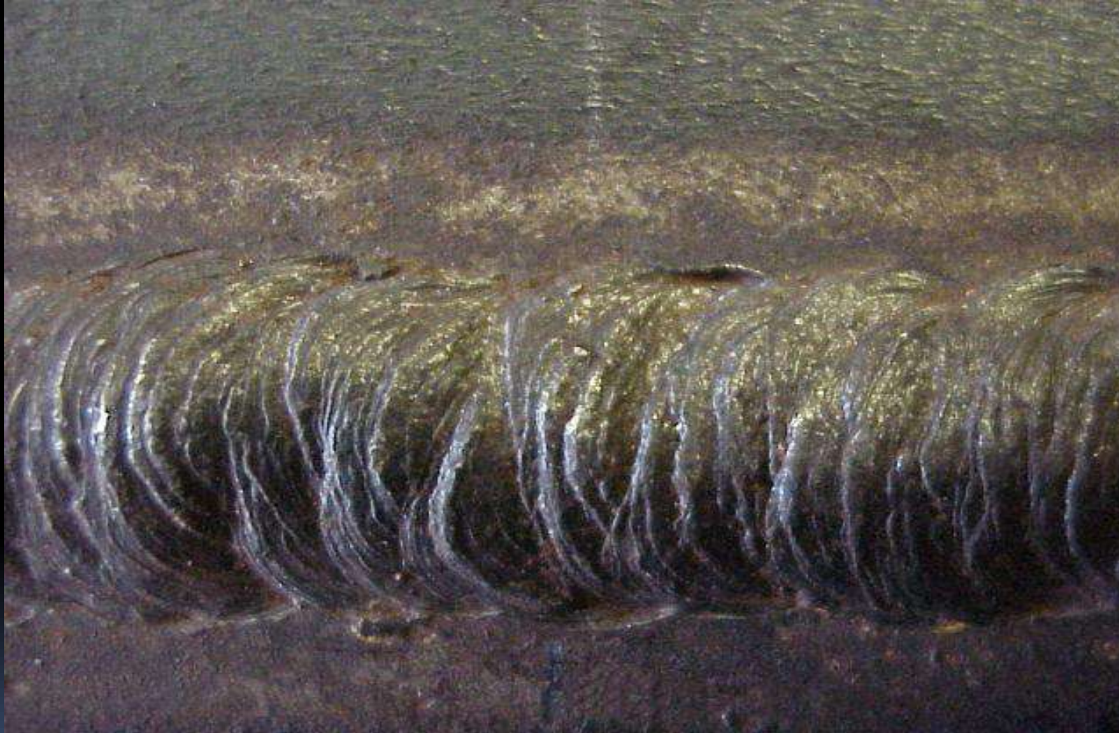
Intermittent Cap Undercut
