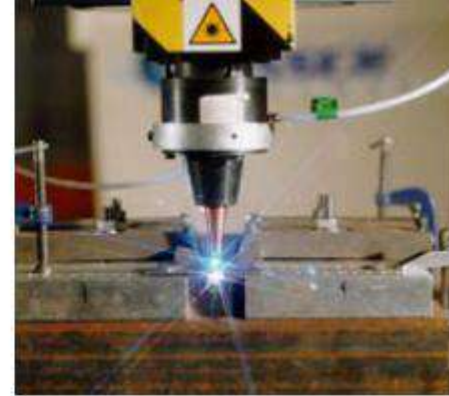
CO 2 laser welding of low carbon steel sheet
