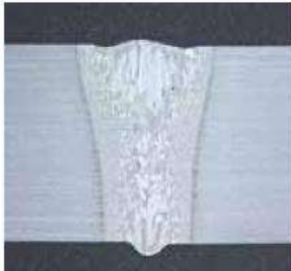
Nd:YAG laser weld in 6 mm thick Ti-6Al-4V
