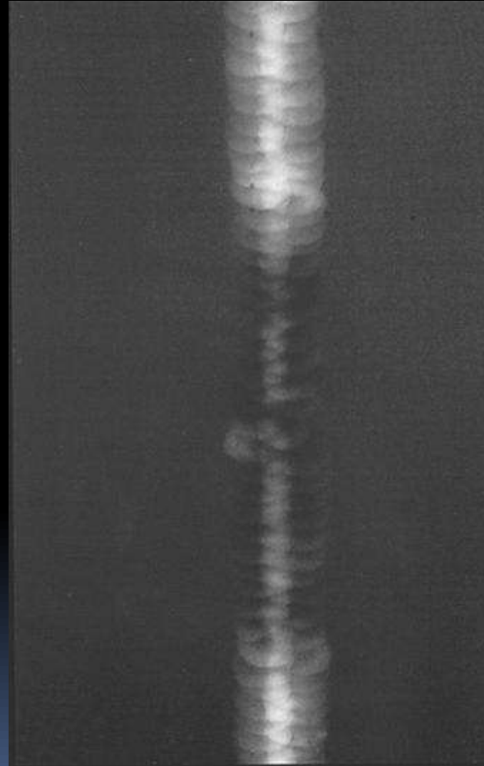
Incomplete filled groove
